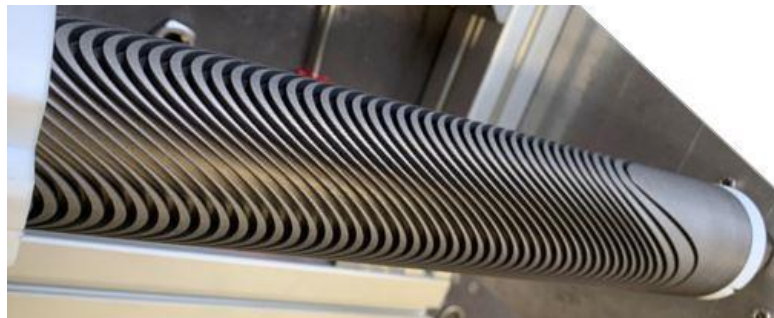
Curved \cos\theta dipole with H-split yoke with assembly clamps - Courtesy Mikko Karppinen, CERN
