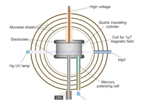
Mercury co-magnetometer (1998)
